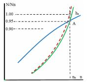
Figure 1 Combined point between Main Engine -Propeller in designing
